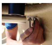
Bolt securing outrigger kit to Bushranger
