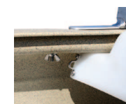
Bolt securing motor bracket to Bushranger
