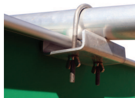
U-Bolt securing outrigger kit to Swagman
