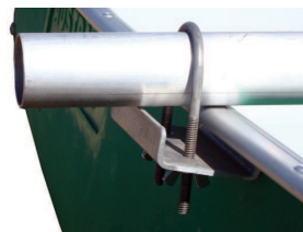
U-Bolt securing outrigger kit to Swagman
